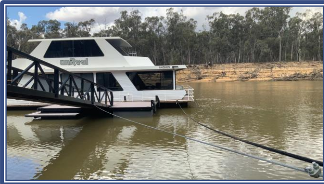
Figure 4-7 – Images showing the Structure tieback point and mooring line (Source PRS November 2024)
